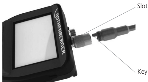
Figure 2 - Cable Connections (Connector Style A, Black Color)
