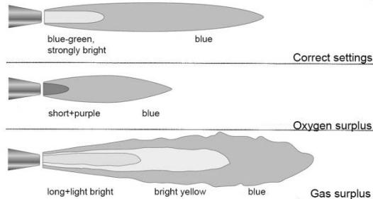
Then set to a neutral flame. This means that the strongly glowing blue-green core of the flame must be sharply delineated from the blue border of the flame (the secondary flame).
